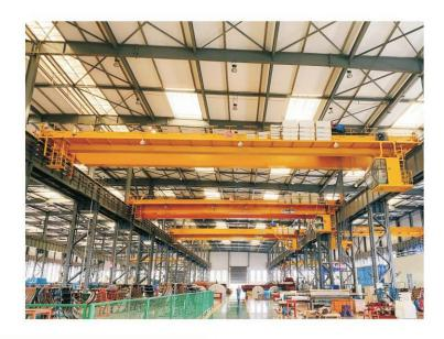
Overhead crane is the hoisting equipment that stands across workshop, warehouse or stock ground to hoist materials. And its two ends are located on high concrete column or metal support. Also known as the bridge crane, it runs longitudinally along a track with rails laid on the elevated support on the two sides.
