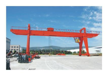
Gantry crane is also called as frame crane, which is mainly being used for loading and unloading materials of outdoor yard and stock ground. It can walk on the track of the ground directly and have the outriggers on the two ends of girder.
